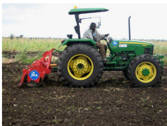
Photos 1.5: Soil clod crushing by rotary Photos 1.6: Crushed soil clod after two times by rotary cultivation (no soil clod of more than 4 cm)
